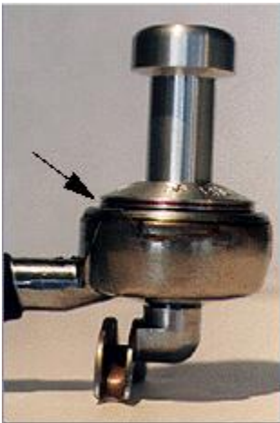
Fig. 2: "Ergo-packer" features engraved lines to check the dosage and level-ness of a pack.
